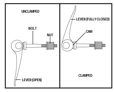
Figure 18. Quick Release Fastener Operation
